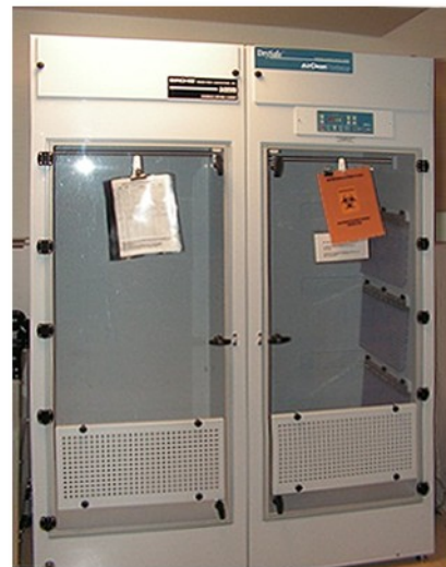
EXAMPLE 2B: Blood Drying/Wet Evidence Drying Equipment
