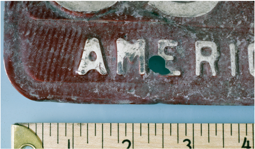
Fig. 20-1 Fabric impression on a license plate from a hit-and-run investigation.
