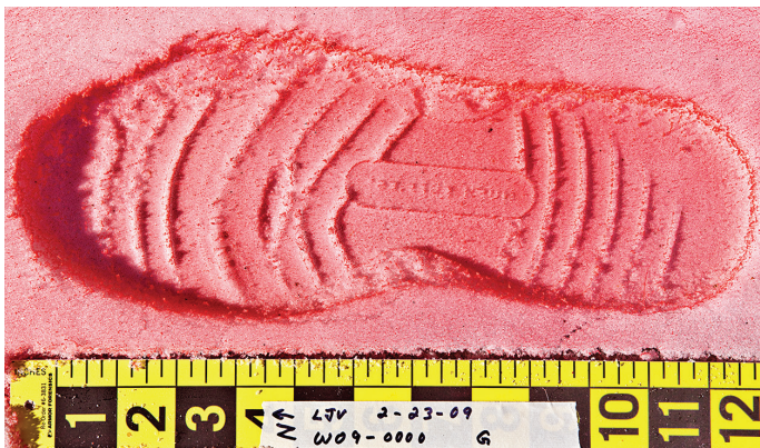
Fig. 10-4 Impression sprayed with snow print wax which enhances detail of impression and creates a buffer for the dental stone.
