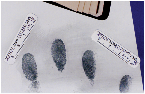
Fig. 2-19 This is what is meant by filling the viewfinder with the evidence (latent prints) and the ruler when using film and adequate resolution digital cameras.
