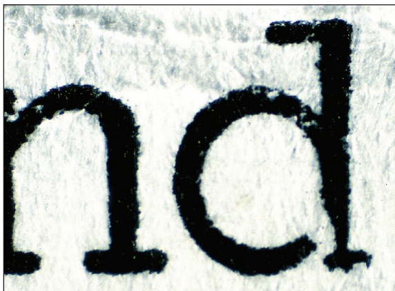
Fig. 33-5 Typewriter defect in an anonymous bomb threat.
