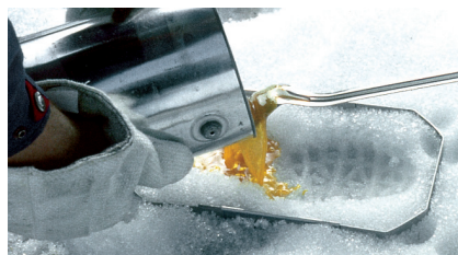
Fig. 10-12 Sulfur mixture is poured into the footwear impression using a deflector (metal spoon).
