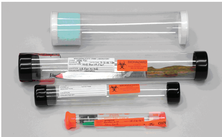
Fig. 1-3 Examples of plastic sharps containers. Do not package knives in plastic containers if DNA testing is requested.
