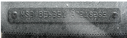
Fig. 2-6 The flash was moved from inside to outside the windshield to side light the VIN number plate. Compared to Figure 2-5, this results in the dust and contamination on the windshield being more visible.
