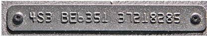
Fig. 2-5 If the VIN plate is mounted on top of the dash, side light it with the flash inside the windshield. Because of contamination on the windshield, you may have to manually focus your lens. The condition of the windshield for Figure 2-6 was the same.
